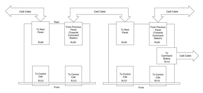
The panel utilises two RJ12 connectors on the face to plug into either side to control trains, two RJ45 connectors on the rear to connect to other panels and an RJ12 connector on the side to connect to the Command Station.
